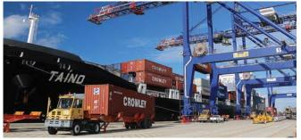
The second of Crowley Maritime's new combination container/roll-on roll-off "ConRo" ships – M/V Taíno, one of the first of its kind to be powered by liquefied natural gas
