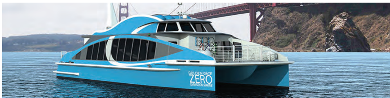
Water-Go-Round | 18m Hydrogen Fuel Cell Catamaran Passenger Ferry | Project Supported by “California Climate Investments” (CCI) program
