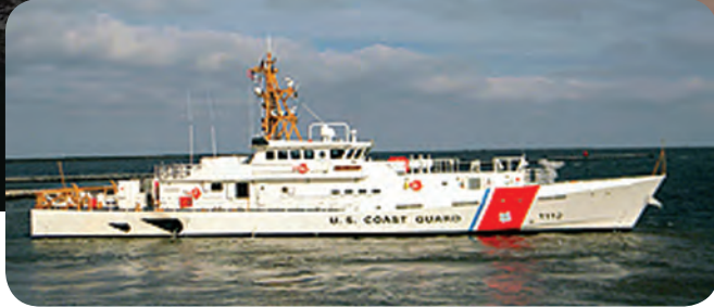
USCGC ISAAC MAYO during trials in the Gulf of Mexico; Courtesy of Bollinger Shipyards. The FRC is based on the Damen's Stan Patrol Boat 4708 design.
