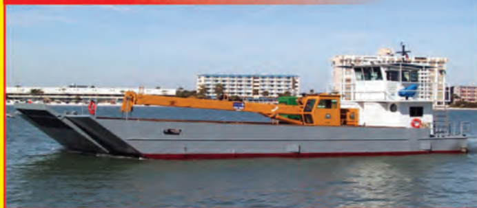
70' Landing Craft w/30ft Beam & Deck Ramp
