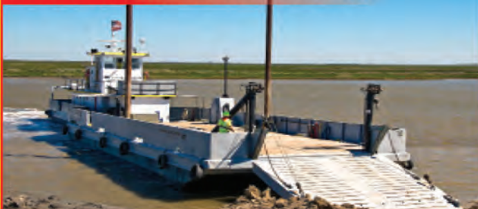
115' ITB - Twin 225HP Detroit Diesel 6-74's NA
