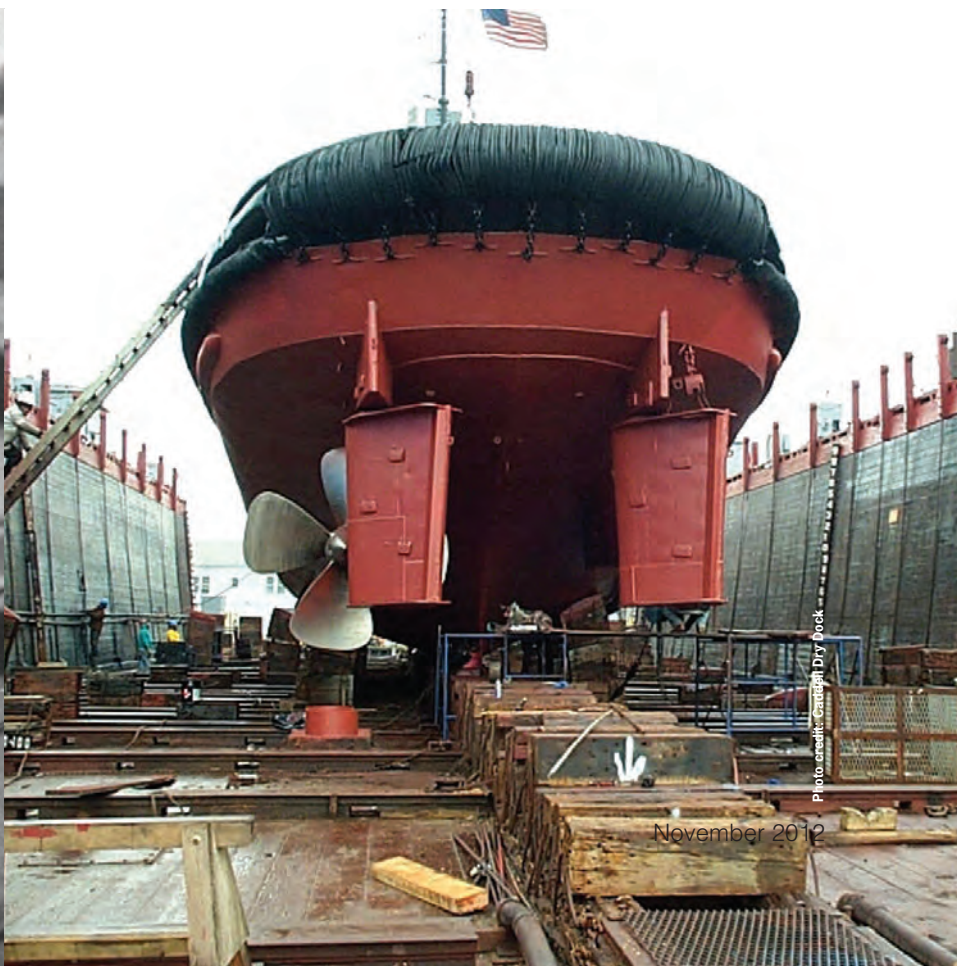
RIGHT Tugboat in a dry dock for hull painting and propeller work at Caddell Dry Dock & Repair Co.
