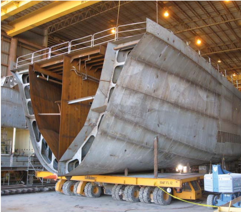
The hull of Crowley's Ocean Class tug under construction at Bollinger Shipyards in Louisiana
