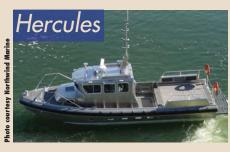
225 nautical miles. The vessel's cabin features sound deadening material keeping the decibel range in the low 70s while running full power. Shock mitigating seating and flooring reduce crew fatigue for longer range patrols.
