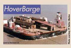
sands of tonnes in payload over swamps, tundra, ice and shallow water. A significant advantage of the hoverbarge is that it only exerts one psi ground pressure while on hover, thus minimizing any environmental footprint.
