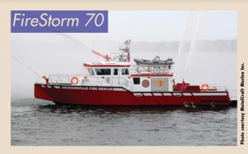
speeds of 41 knots with four CAT C-18s at 1,015 hp each. Ships electronics are Furuno 3-D system communications by Motorola ICOM & Piratecom. The wireless Piratecom can interface with up to six radios and cell phones and has wind and engine filters for audio ability.
