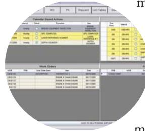
offshore oil and gas workboat industry. Preventer is an add-on module to SAMM that provides automated, company-specific preventive maintenance procedures, safety inspections and any other maintenance or inspection routines required on a vessel. Preventer captures and schedules procedures through an intuitive, scalable and customizable application.
