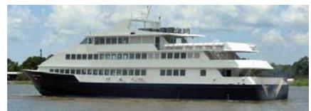
Conrad Industries delivered an aluminum passenger vessel for Puerto Rico Maritime Transportation Authority (PRMTA). The Cayo Blanco can carry 600 passengers on two decks and measures 160 x 32 x 13 ft and is powered by four MTU 12V-4000 M60 main engines with MGX 6848 Twin Disc gears. The generators are John Deere and there is a 200 hp tunnel bow thruster.
