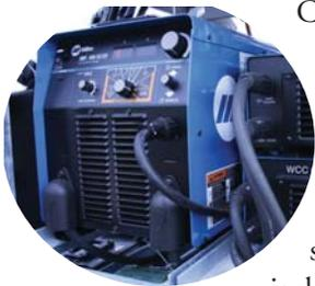
This MIG/Flux Cored welding system allows welders in the construction and shipbuilding industries — who often work more than 100 ft away from the welding power source — to adjust voltage settings at the point of use.
