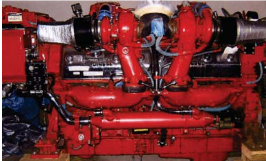
12 Cylinder Detroit Diesel Model 12V149TIDDEC 1800 HP @ 1900 RPM Heat Ex. w/2.5:1 Gear, Low Hours- $66,000 Each
