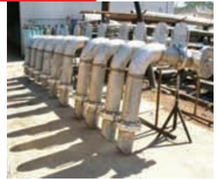
FABRICATION OF STAINLESS STEEL MANIFOLD
