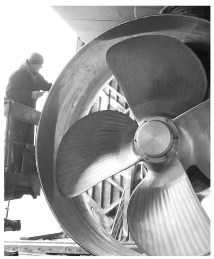
It takes a big propeller to move a tug against an LNG tanker underway. The pair on the Edward J. Moran are attached to Rolls Royce US 255 Z-drives, driven by two EMD 12-710-G7B main engines, bollard pull given as 176,760 libs. ahead, 170,000 astern. (Photo: Don Sutherland.)
