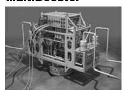
The MultiBooster subsea multi-phase pump system designed to deliver improved oil recovery and facilitates longer step-out distances between subsea assests and host facilities by lowering pressure at the reservoir and increasing pressure in the production line. Under development since 1998, the system utilizes twin-screw internals and Aker Kvaerner's pressure-volume regulator to provide a flexible and robust subsea solution.
