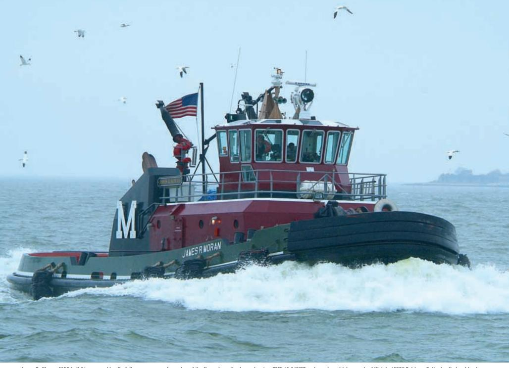
James R. Moran, W&D hull 81, approaching Norfolk one year ago. A member of the Kaye class, the James has two EMD 12-645f7B main engines driving a pair of Ulstein 1650H Z-drives. Bollard pull ahead is given as 139,000 lbs; 135,000 astern. (Photo: Don Sutherland.)
