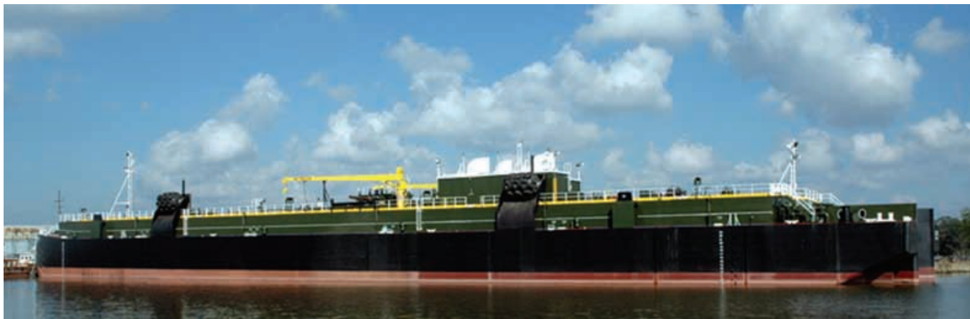
K-Sea's new 103,000 barrel double-hulled barge along side the dock at Bollinger Marine Fabricators, Amelia, La.
