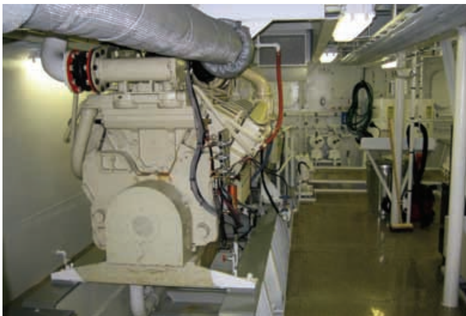
The Norman P. Proehl is powered by a pair of Cummins KTA50 main engines each rated for 1600 hp at 1800 rpm turning a pair of 80 x 64-in. propellers. (Photo: Horizon Maritime)
