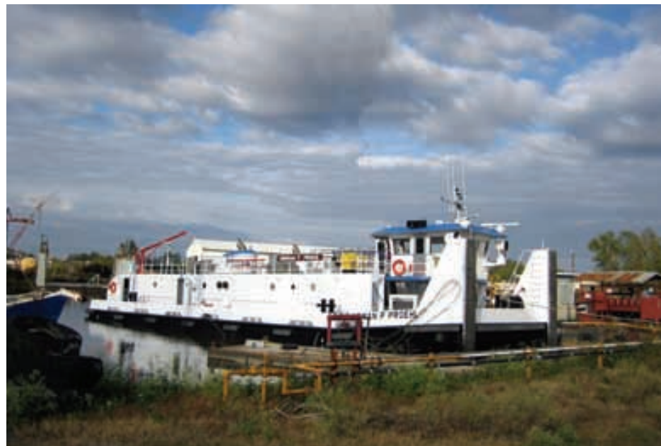
Horizon Maritime has a new retractable wheelhouse towboat, the Norman P. Proehl, that pushes barges along the canals that connect the Great Lakes to the Illinois and Mississippi system south of Chicago. (Photo: Horizon Maritime)
